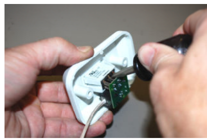
With switch plugged in short from center silver lug to each outside lug. One side should move beds up – the other side down,
