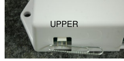
The 3 pin output can be shorted by lacing a paper clip or stiff wire alternately over and under the pins, or shorted with an alligator clip.
