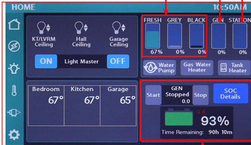
**Note: The AGS system will be disabled when a manual start or stop is detected. A manual start is allowed 90 seconds to complete before suspending the starting process with the error message "Fault". When a manual start is selected the number of retries are set up on the AGS screen.**
