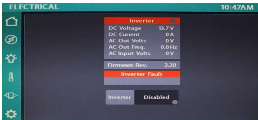
This is the Initial electrical screen if the unit does not have the generator option and has a Progressive inverter.
