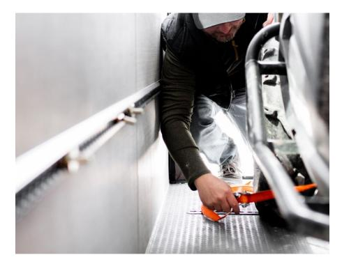
TIE DOWNS Nine floor airline tracks are fastened directly to the frame.
