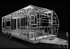
PLĀ\* toy haulers are built to last with a fully integrated aluminum frame. The six-sided "welded box" has no fasteners to loosen over time and features a one-piece aluminum roof. Unlike most other toy haulers, there is no wood in our construction to rot and deteriorate over time. PLĀ toy
